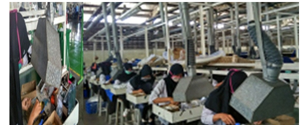
Exhaust systems on the shop floor area in our Indonesia factory
